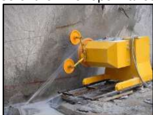
Figure 9: Diamond Wire Rope Cutter
