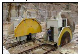
Figure 10: Double Blade Cutter
